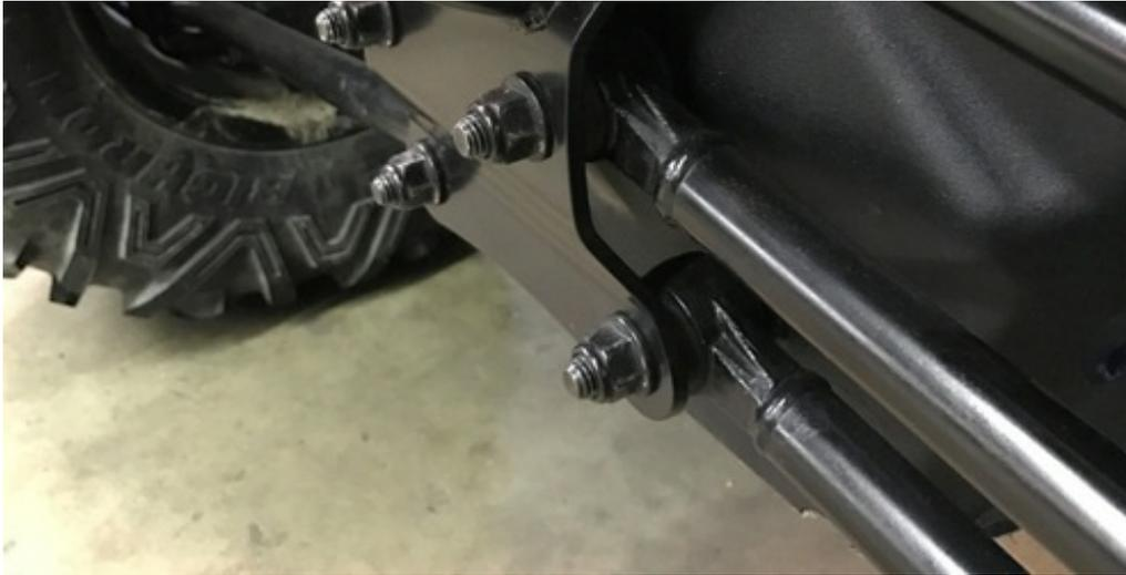
6. Tighten the bolts that connect the 2 top support bars to the top of the bumper.
