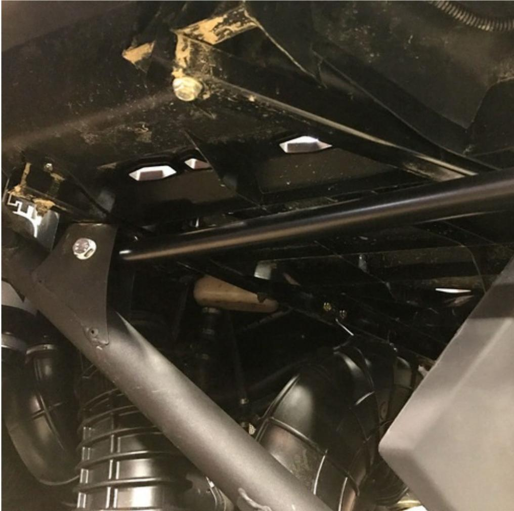
2. Install the rear bumper so that the bottom mounting plate slides over the 6 radius rod bolts.
